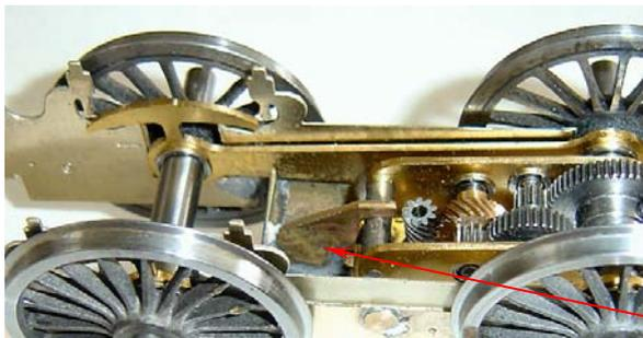
alignment errors will effectively pinch the axle causing drag and premature failure of the gearbox. Most modern motor/gearbox units are small enough to allow a compensation beam beside them. The ideal restraining system will vary depending on the unit you are using but a type of fork in the middle of the chassis hooked onto the gearbox is one solution.
