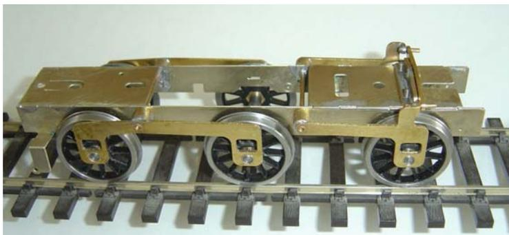
Not everyone compensates the tender as it is not really a part of the locomotive but a piece of rolling stock that always seems to accompany the locomotive. The only exceptions are when the tender is motorised or used to collect electrical current. There are a number of advantages to
