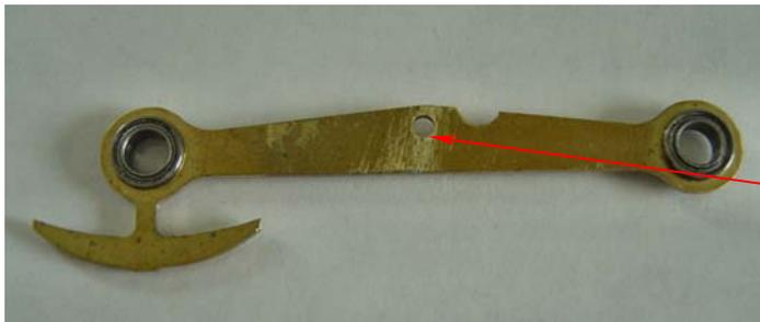
Compensation Beam fitted with ball races. The beam includes a dummy leaf spring and a cut-out to miss the brake gear.
